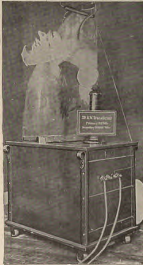
Transformer Discharging Through and Around a Heavy Glass Plate.
